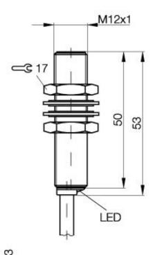
**Inductive Sensors** BES M12MI-PSC40B-BP03 M12x1 x 53 normally-open Sn=4mm shielded
